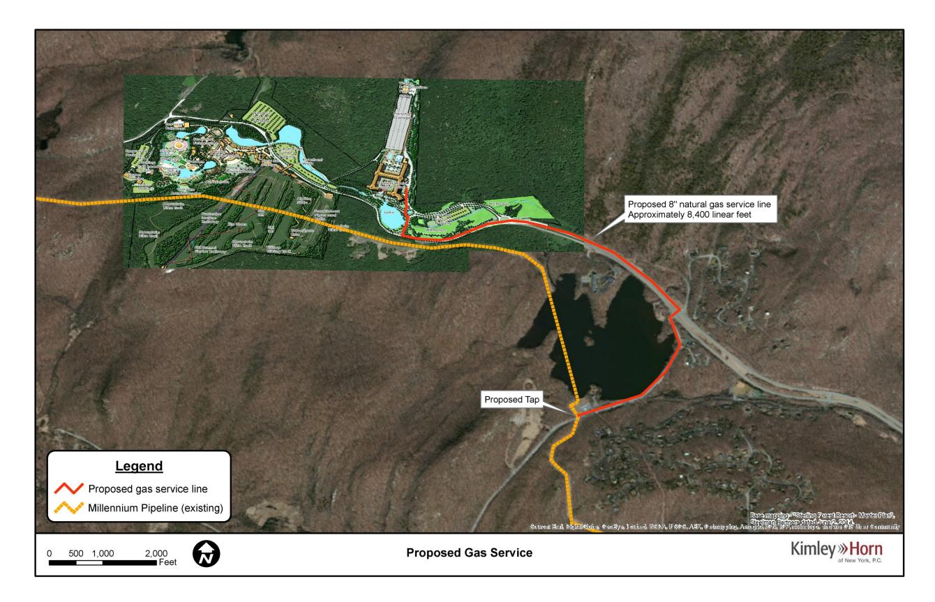
Proposed natural gas infrastructure for Sterling Forest Resort includes a new 8-inch plastic distribution main to be run by ORU from the existing Millennium pipeline tap near Longmeadow Road. The 8-inch line is approximately 2.5-miles long and will be located in the roadway right-of-way of Longmeadow Road and 17A.
