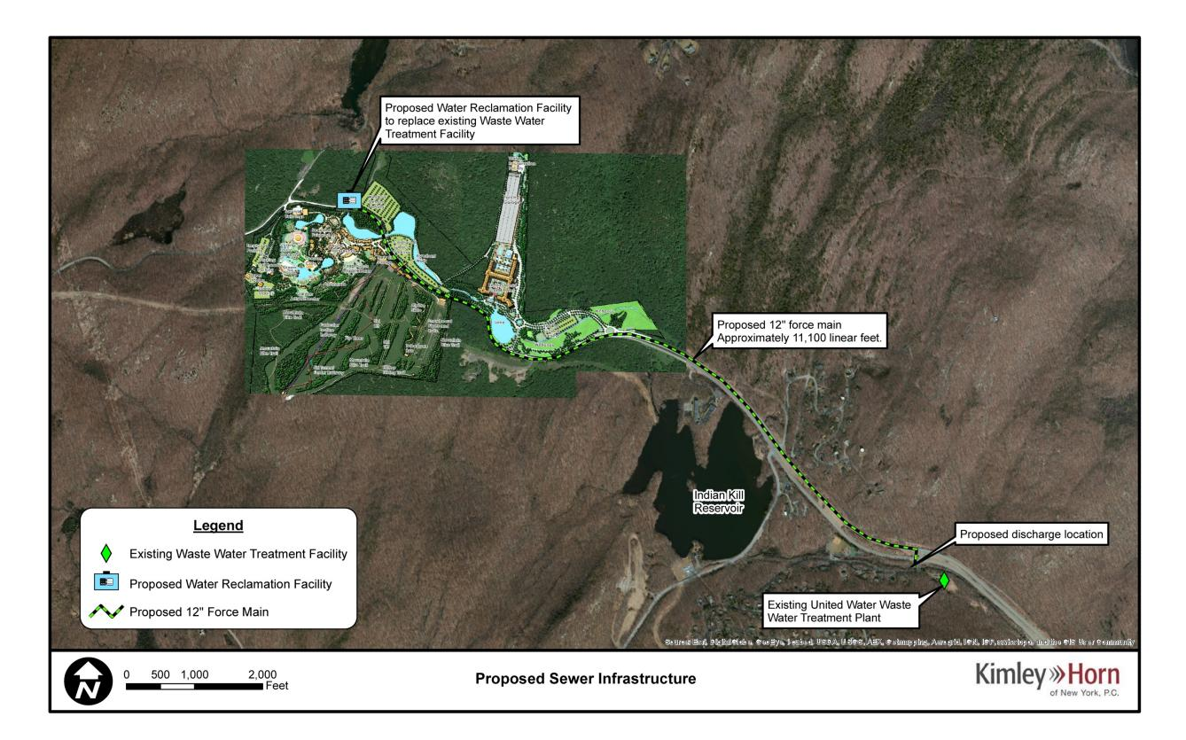
A water reclamation facility (WRF) is proposed for the Sterling Forest Resort. Sewer demand projects were calculated and resulted with an average daily flow (ADF) of 308,500 gpd with a peaking factor of 2.5 and peak flow of 771,000 gpd. The WRF will discharge into the Indian Kill Creek downstream of the Indian Kill Reservoir and will be capable of producing reclaimed water to be used on-site for irrigation, toilet flushing, snow making, and other non-potable uses.
