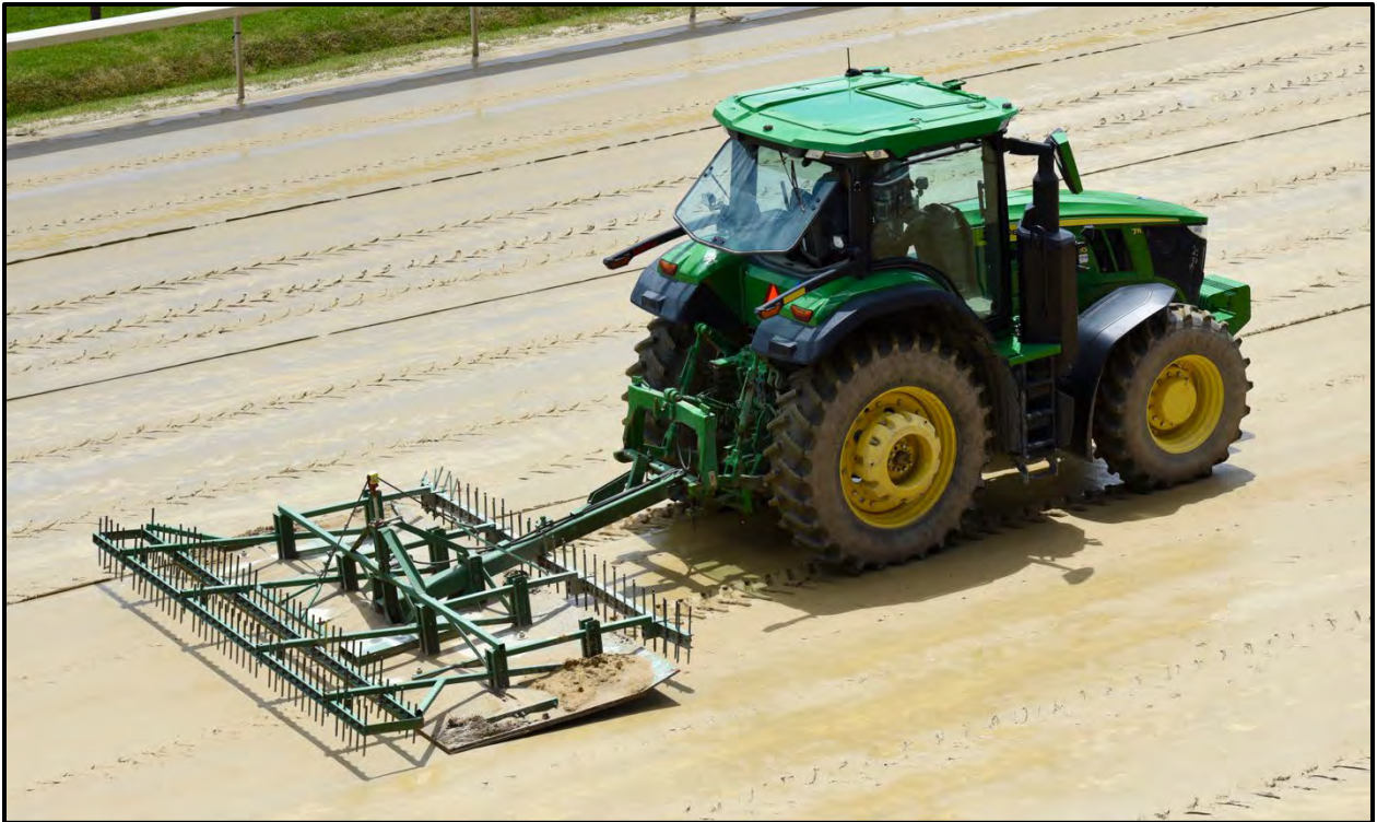
Figure 4. This float is being used to compact and seal the Saratoga Main Track after experiencing approximately ¼ inch of rainfall. (Photograph by Scott E. Palmer)
