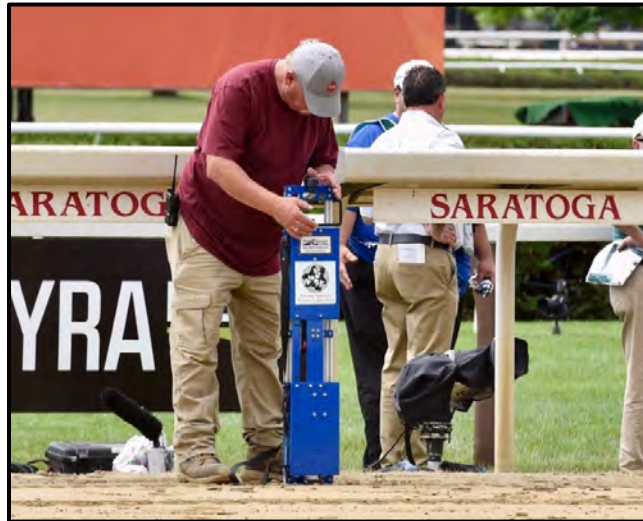
Figure 13. Time Domain Reflectometry (TDR) was used to obtain moisture content data from the Main Track. (Photograph by Scott E. Palmer)
