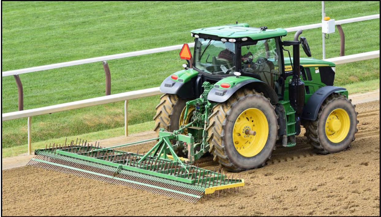
Figure 2. Harrow being used on the Saratoga Main Track to smooth the surface and remove hoof prints. In this image the back rake has been lowered to provide a second layer of teeth to further smooth the surface. (Photograph by Scott E. Palmer)
